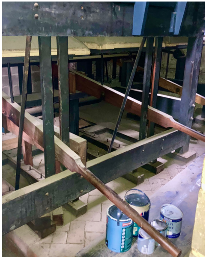
The whole rocker mechanism of the bellows can be seen
