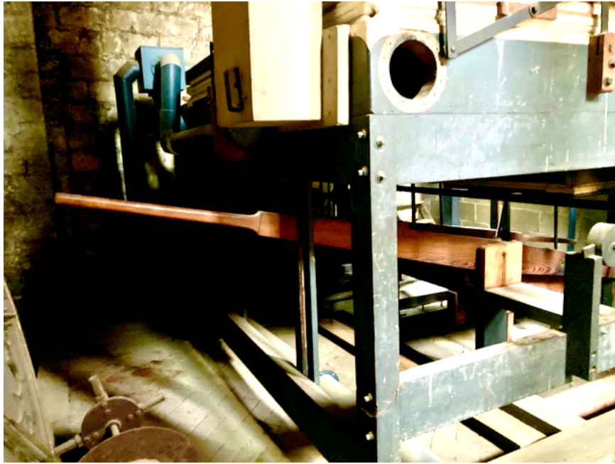
One of the rocker arms on the manual bellows
